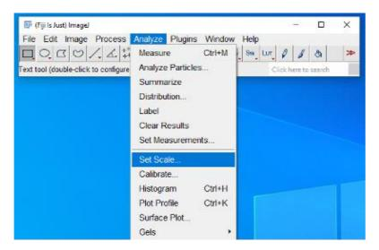
Then specify a known width in both pixels and physical distance and a measurement unit (i.e.  $\mu m$ ). This is where knowing the HFW comes in. You may specify the HFW as the known distance, and the pixel distance is just the number of pixels wide the image is (i.e. 1536 is the default for the photo preset in the Helios microscope):
